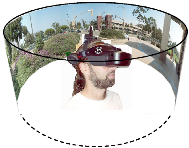
Fig. 3. Illustration of how the computer simulates the location shown in Fig. 2. The panoramic photograph is applied to the inside surface of a computer-modeled cylinder. The user’s viewpoint is then placed in the center of the cylinder.
