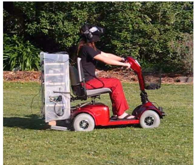
Fig. 8 Electric vehicle with onboard PC, tracking sensors, and Virtual Research V8 head mounted display provided wireless, mobile virtual reality motion base simulator. Participants performed the lane change and path following conditions both with and without visual feedback. However, they also have inertial information due to real movement of the vehicle
